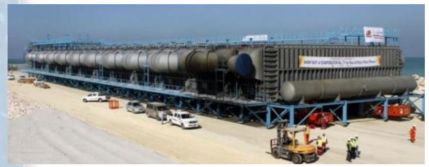
This evaporator measures almost 124 meters long, 34 meters wide and 12 meters high, the evaporator weighed in at a mammoth of 4,891 tons. In size, It is equivalent to a football field and with an assumed weight of 5000 cars. This evaporator is destined for Saline Water Conversion Corporation's (SWCC) in Ras Al Khair Power and Desalination Plant Project.
